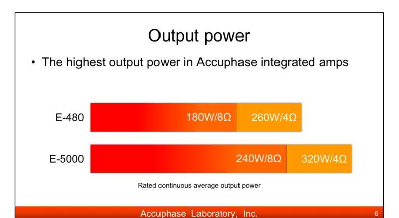
The E-5000 has the highest output power in Accuphase integrated amps, the rated continuous average output is  $240W/8\Omega$ .
