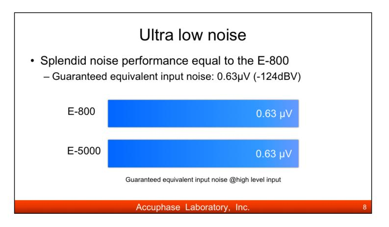
The E-5000 realizes -124dB (  $0.63\mu V$  ) of equivalent input noise equal to the flagship class-A integrated amp E-800.
