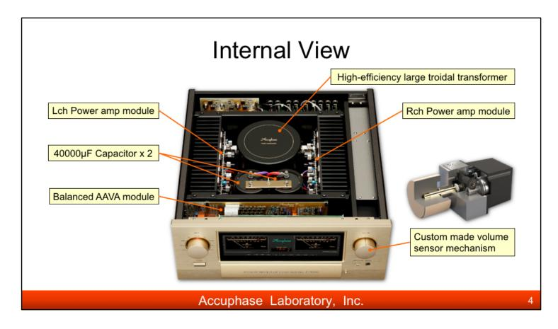
E-5000 has the mono-block construction. The strong power supply with massive, specially-made and high-efficiency toroidal transformer and 40000µF filtering capacitors are installed in the center of the unit. In addition, the two power amplifier modules are kept separate for the left and right channels.
