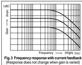
Fig. 3 Frequency response with current feedback (Response does not change when gain is varied)
