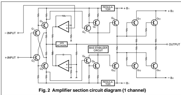
Fig. 2 Amplifier section circuit diagram (1 channel)
