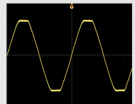
Photo (b) Voltage waveform of AC line (distortion approx. 3%)
