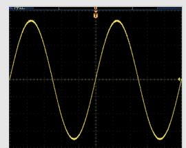
Photo (c) PS-510 output waveform (distortion approx. 0.2%)
