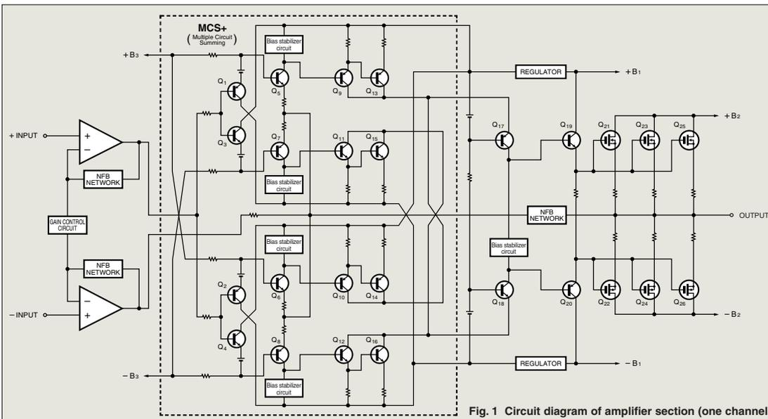
Fig. 1 Circuit diagram of amplifier section (one channel)
