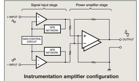
in excellent CMRR (Common Mode Rejection Ratio) and minimal distortion. Another significant advantage is that external noise and other external influences are virtually shut out. The result is a drastic improvement in operation stability and reliability.
