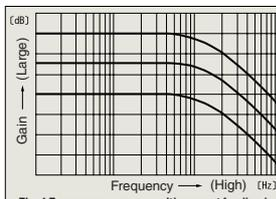
Fig. 4 Frequency response with current feedback (Response remains uniform also when gain changes)
